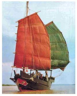
from Fukien (Fujian) north to Chekiang (Zhejiang) have round oculi. They are typically made of two painted wooden circles sandwiched on top of each other and mounted on both sides of the bow. Fishing vessel oculi focus downward to help fishermen search for fish and scare away competitors such as whales, while trading vessels gaze forward, helping to navigate clear passage ahead.
